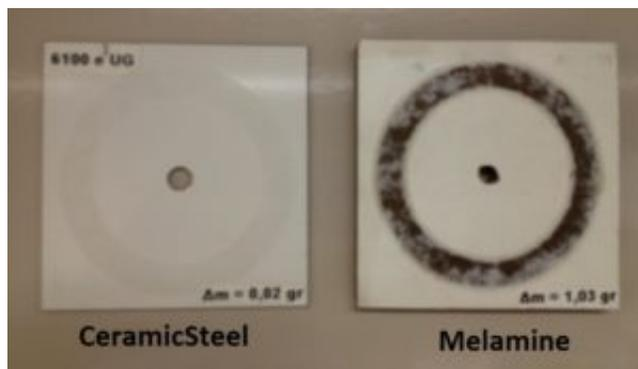
CeramicSteel shows very little abrasion, while dry erase paint is eroded to the substrate. This shows that whiteboard paint will not maintain its quality in areas with heavy traffic and will not withstand long-term use. Over time, the surface will degrade and require re-painting or replacement. e3 CeramicSteel will never decrease in erasability and the surface will not wear away over time.
